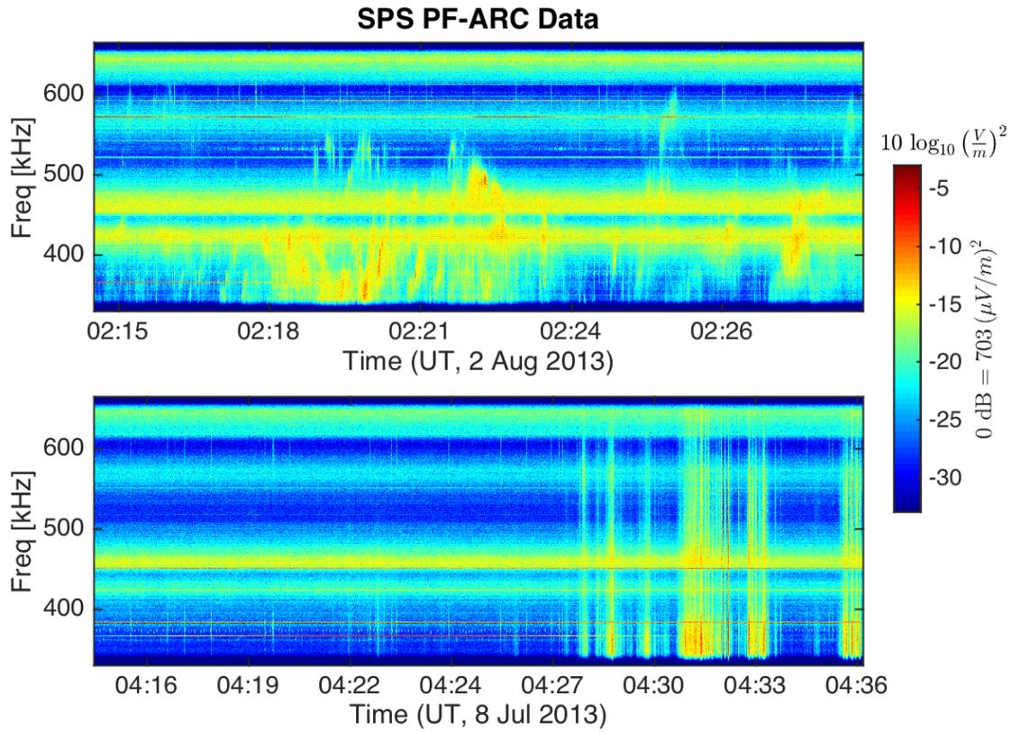
**Figure 6.** Results from the PF-ARC at South Pole Station. The upper spectrogram shows fine structures in signals which appear similar to Auroral Kilometric Radiation, while the lower plot shows an example of auroral hiss, for comparison.
