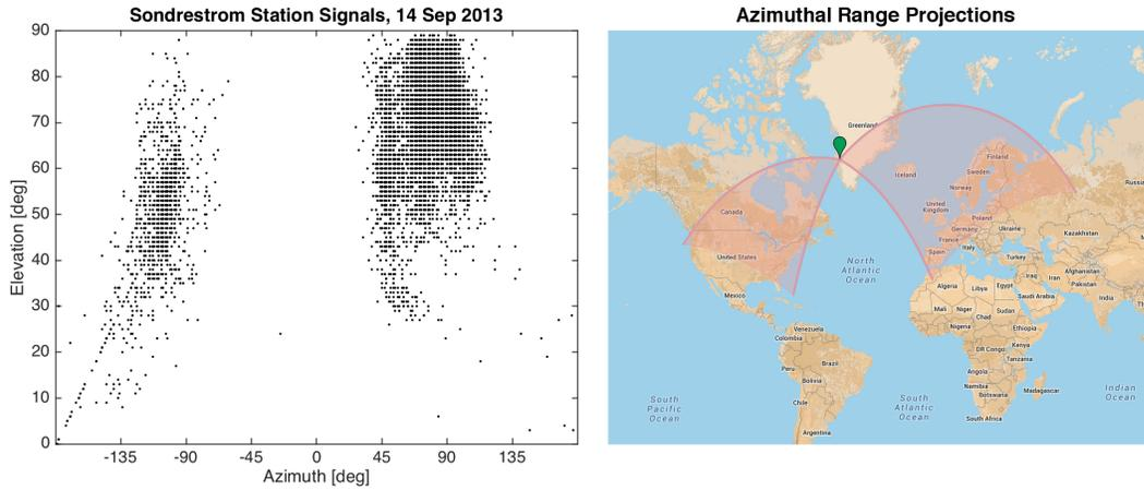
**Figure 7.** Proof of functionality for the MI-ARC at Sondrestrom Station. To the left, an elevation vs. azimuth scatter plot (elevation from the horizon, azimuth in degrees from true north) of high-coherence points for 14 Sep 2013, showing two clear clusters of points. To the right, we project the azimuthal ranges of the two clusters onto a map, implying that the clusters correspond to signals transmitted from Europe and North America [Map data ©2015 Google, INEGI].
