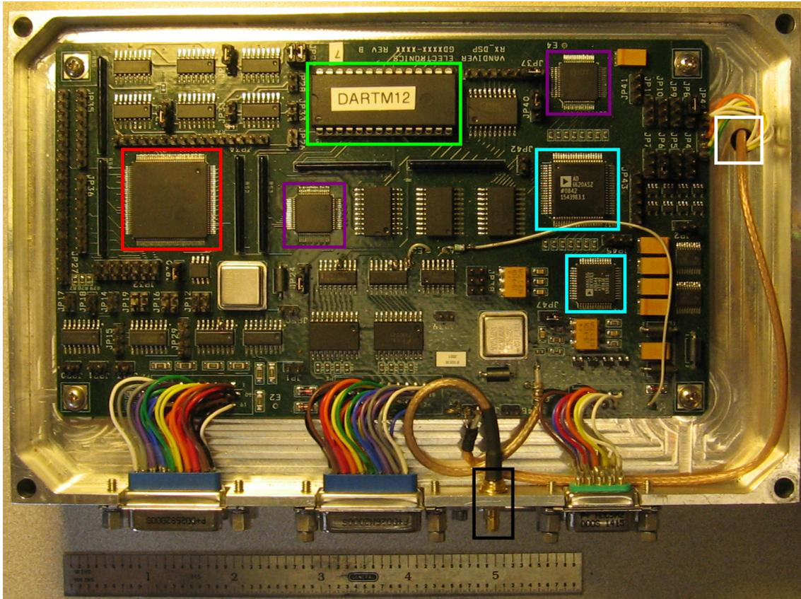
**Figure 1.** A photograph of the top board of an Rx-DSP stack ready for a rocket flight, with 6 inch ruler for scale. Highlighted are the SMB signal input (black), cross-board synchronization lines (white), AD6644 & AD6620 signal processors (cyan), IDT72285 FIFOs (purple) TMS320C542 programmable processor (red), and the program-code EEPROM (green).
