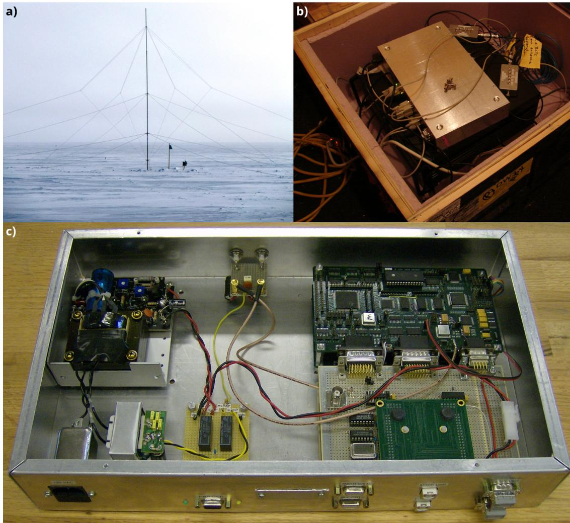
**Figure 5.** Photos of the various components of the South Pole Station PF-ARC. Top left shows the crossed-loop antenna with a 30 ft mast, and the pre-amplifier at the base. Top right shows the receiver box, data-acquisition PC, and various other equipment within an insulated box (covered when in operation). Bottom shows a lab-bench photo of a PF-ARC, with two vertically stacked, sample-synchronized Rx-DSP boards and adjoined QuickUSB breakout boards on the right side.
