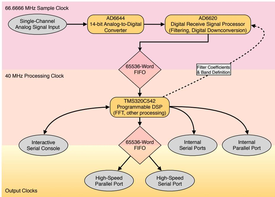
**Figure 2.** A diagram depicting the major parts of the Rx-DSP hardware, and the data flow between them, with the dashed line indicating command/control and solid lines indicating data or both. The colored background boxes indicate which systems are controlled by which clocks.
