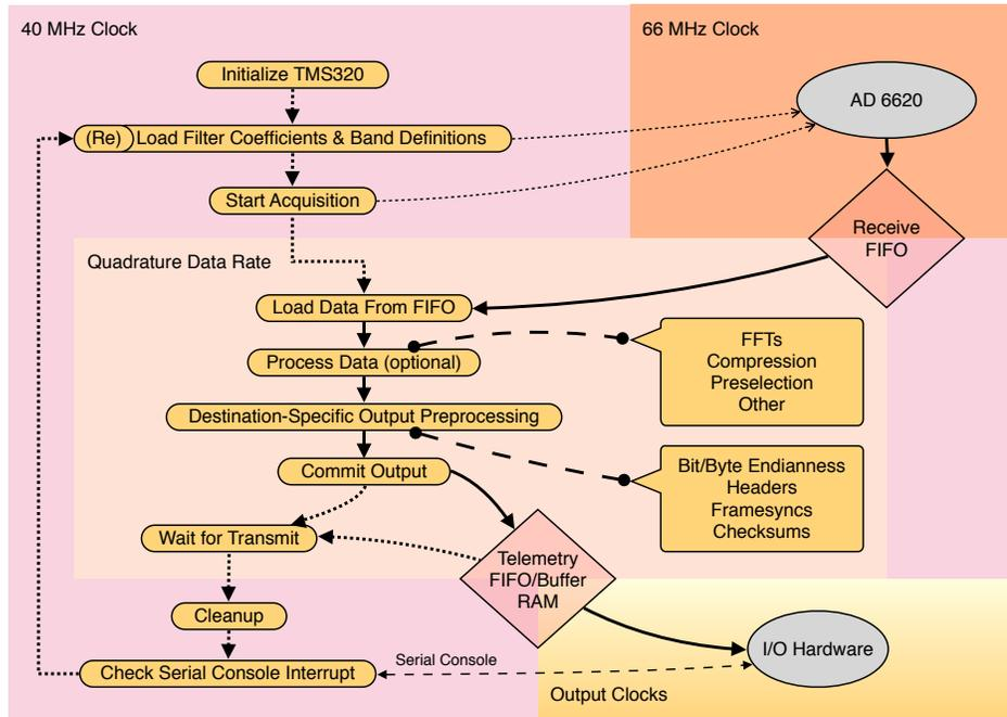
**Figure 3.** A diagram depicting a generalized program flow for the Rx-DSP assembly code. Dashed lines indicate command/control flow, while solid lines include data as well. Color backgrounds show which parts of the code run at the given clock rates, with FIFOs and wait cycles allowing for asynchronous operation. The two callout boxes show modularized routines in the codebase, some, all, or none of which may be used by a given ARC.
