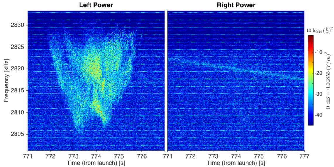
**Figure 4.** Power spectra of Rx-DSP data from CHARM II, recombined to yield left- and right-circularly polarized powers. The line of power with decreasing frequency seen in the righthand plot is an interference line of unknown origin which exists through much of the flight, and has been seen on other flights.
